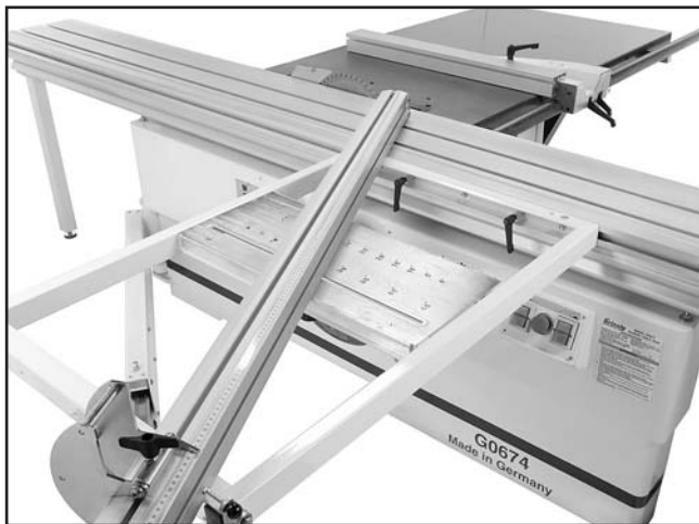
Figure 73. Fence set-up for 90° to 135° cuts.
